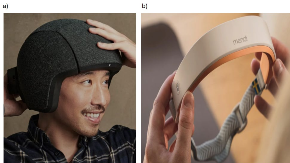
Figure 2. The Kernel Flow and Mendi headsets use fNIRS technology
